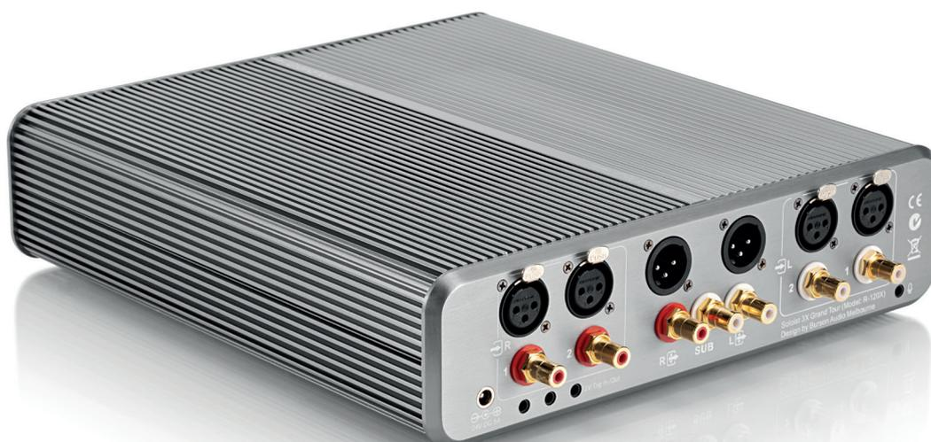
► amplifier terms, with a capital G. The output of 10 Watts per channel into a 16 Ohm XLR load and 640 mW into 600 Ohms is more than twice that of some of its competitors. Output halves if the single-ended TRS socket is used.
