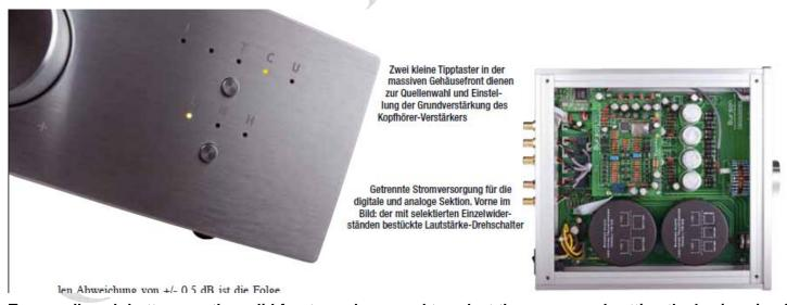
Two small push-buttons on the solid front panel are used to select the source and setting the basic gain of the headphone amplifier
